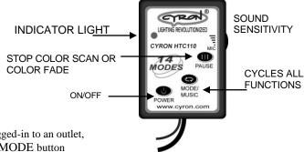
System ON when power is supplied: With the system still plugged-in to an outlet, turn the unit off using the POWER button. Press and hold the MODE button for 3 seconds. Turn the controller on. Now the unit will turn on automatically
