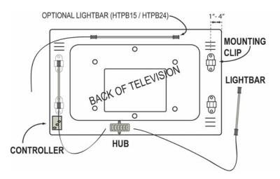
**2** *Connections* Connect all lightbars to the *Media Highlighter* TM system hub. Secure extra cables.
