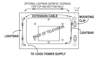
Wiring Lightbars can be connected in series as shown in the wiring diagram. It is recommended to use no more than three lightbars in series to avoid dimming down the line.
