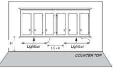
Hub and controller can be placed inside cabinets or above cabinets if space is available.
